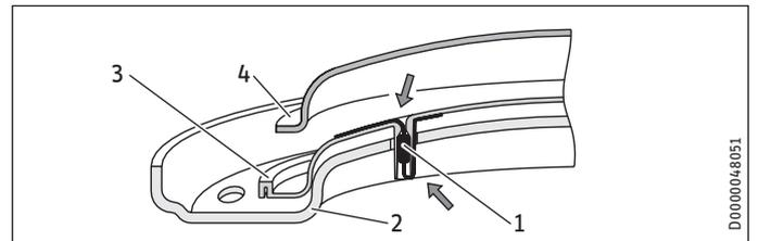
1 Anti-corrosion protection (390 Ω)
