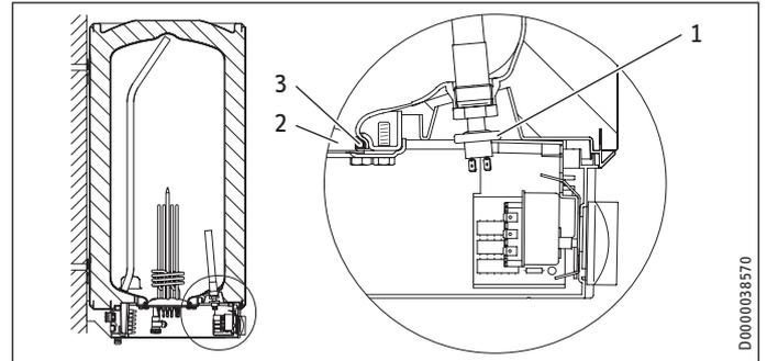
1 Pressure switch for signal anode
