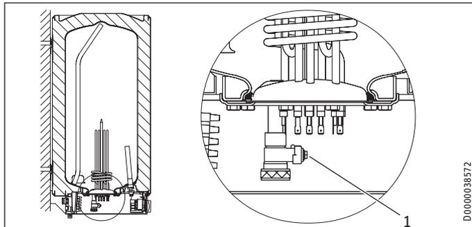
1 Drain valve with hose connection G 3/4
